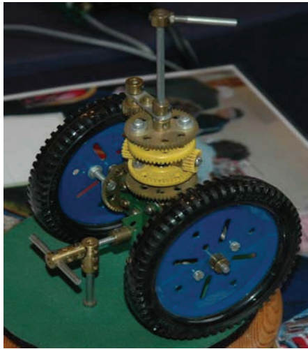
The ever popular South Seeking Chariot was Dennis Backler's model. Details are in the January 1957 MM.
